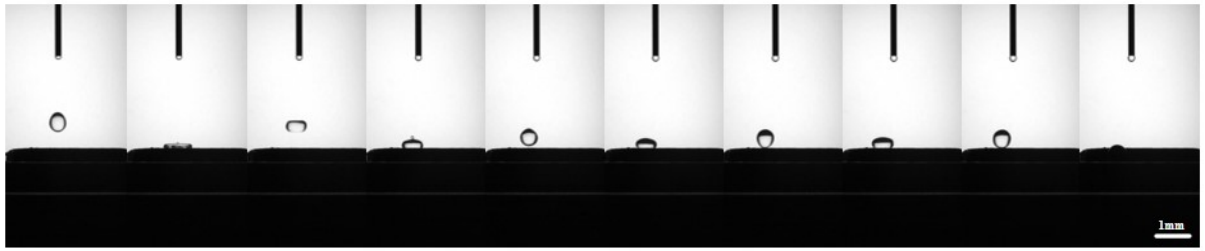
Fig. S5 Bouncing experiment of 50 \mu L droplet on Candle@BC surface.
