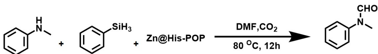
Scheme S4: Schematic representation of N-Formylation reaction by using Zn@His-POP as a Catalyst.
