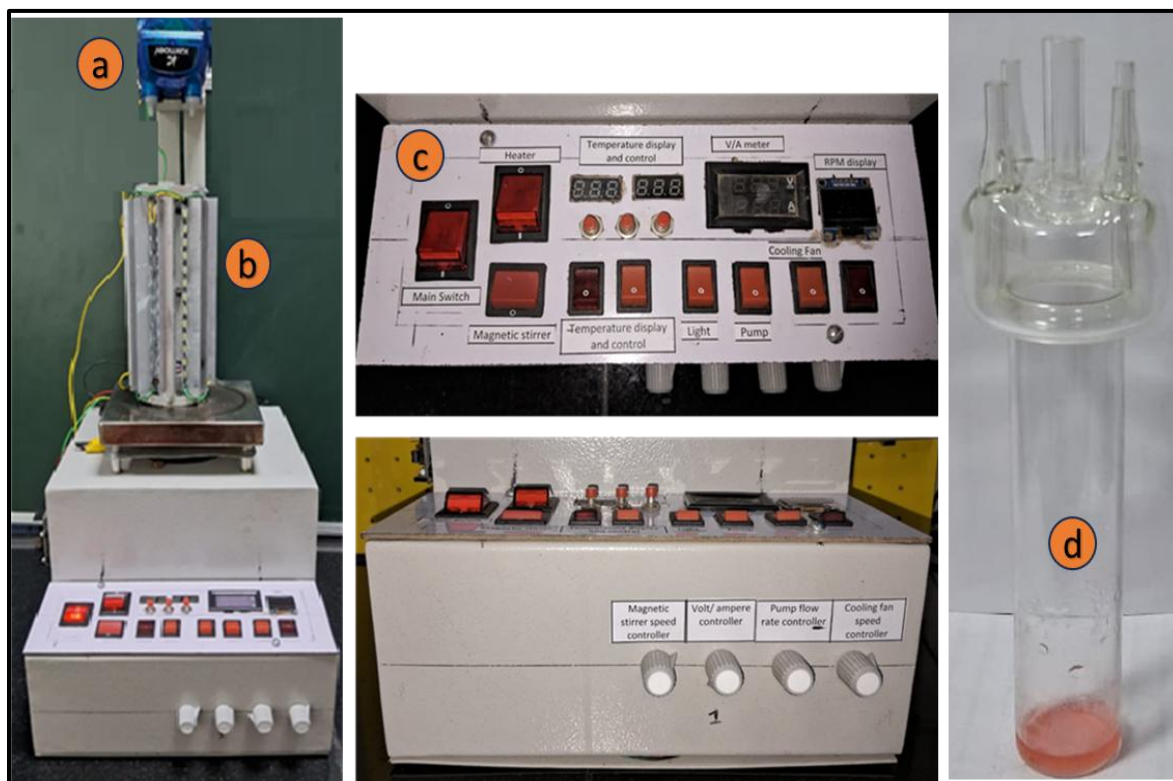
Figure S1. Falling film looping photoreactor consisting of a) pump module, b) irradiation module, c) controller module, and d) reactor module.
