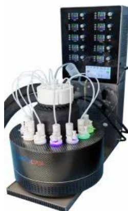
Figure S1 The WP-TEC-1020SL photochemical reaction system with the blue light LED
