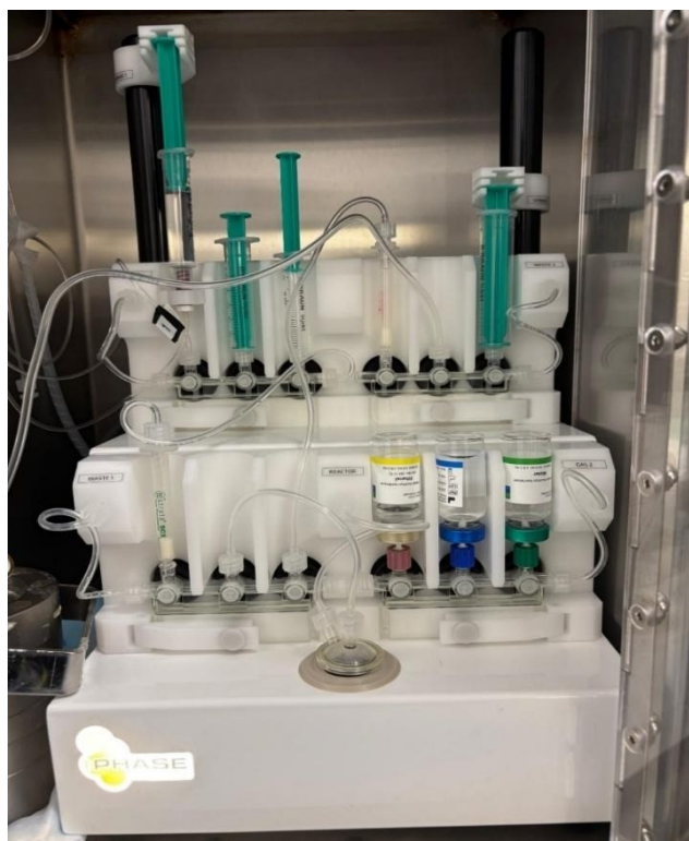
Figure S20 iPHASE MultiSyn set-up for automated radiosynthesis of ^{68}\text{Ga} -PSMA-617.
