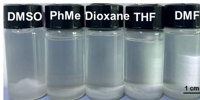
Fig. S9 Dissolution experiment of IEM-DtBIM-0.25 in different solvents at room temperature for 45 days.
