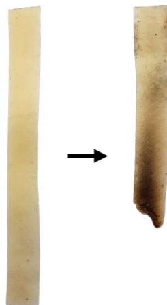
Figure S 22. Gel composite specimen before and after flammability test.
