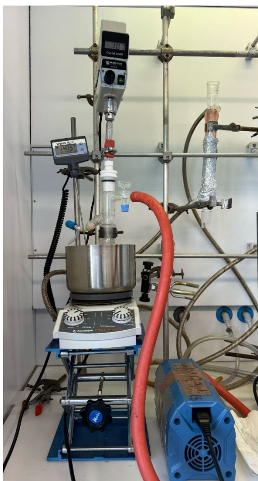
Figure S25. Experimental setup for polycondensation reactions
