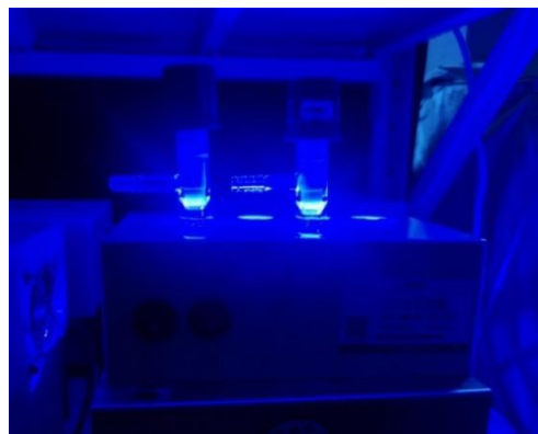
Figure S1. The reaction setup of photocatalytic ATRP polymerization with 6 W blue LEDs ( \lambda_{\text{max}} = 460 \text{ nm} ).
