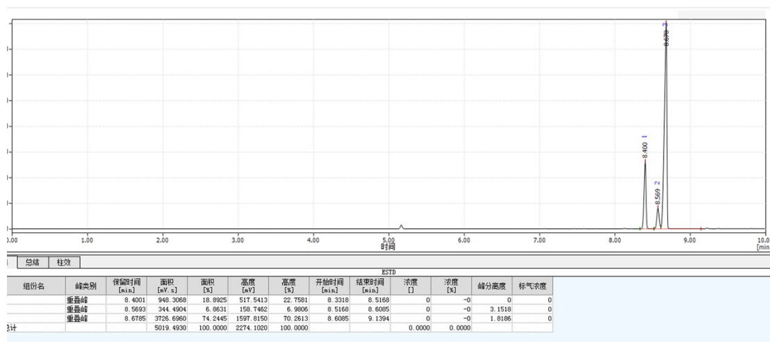
Figure S1. The GC spectrum of VBAMA isomers mixture synthesized in this work
