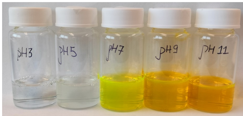
Figure S17. Visual comparison of linear P(OEGMA 6.5 - co -DEGMA 82.3 - co -FluA 11.2 ) solubility/behavior in solutions of varying pH (3, 5, 7.4, 9, and 11).
