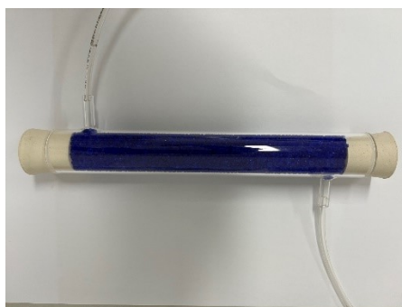
68 Fig. S15. Photographic image of the dehumidification apparatus.
