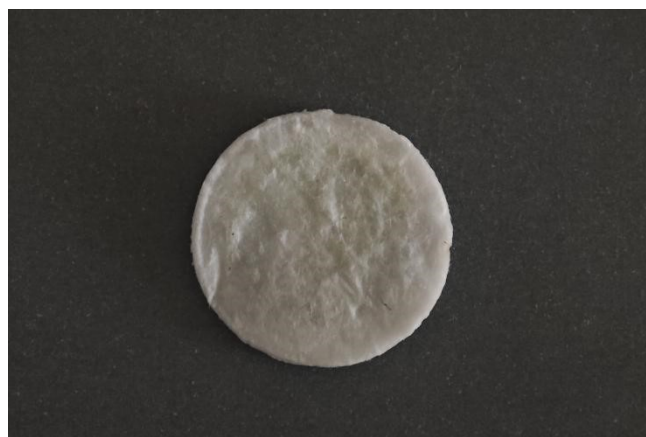
Fig. S5 The morphology of the separator after 150 charge/discharge cycles.
