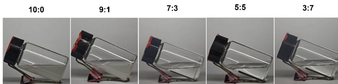
Fig. S3 The solubility data of 0.1M LiNO 3 in electrolytes with different volume ratios of TMM to DOL
