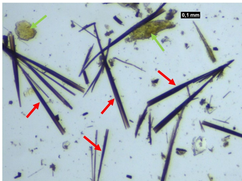
Figure S 4. Microscope picture of the crystals obtained from the solvothermal electrocrystallization of 1\text{-Cd}_2 (red arrows : crystalline dark needles of 1\text{-Cd}_2 ; red arrows ; yellow 1\text{-Cd}_2(\text{TBA}) : green arrows).
