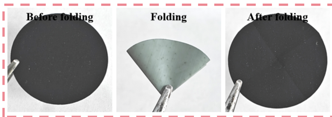
Fig. S15. The folding process photographs of the V 34 -DODA modified separator.
