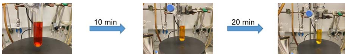
Figure S115. The colour change of the solution of 11 in THF under a CO 2 atmosphere (1 atm) within 20 min.
