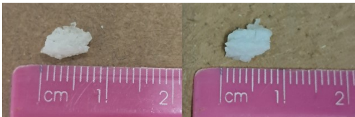
Figure S5. Pictures of poly-PETMP-Ca before (left) and after (right) exposure to an environment of 90% RH and 25 °C for 24 hours.
