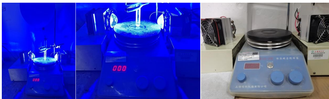
Fig. S1 LED reaction setup for photocatalytic reactions.
