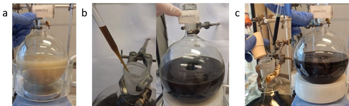
Figure S6. a) reaction quenched too early, b) reaction quenched in time, c) reaction quenched too late.
