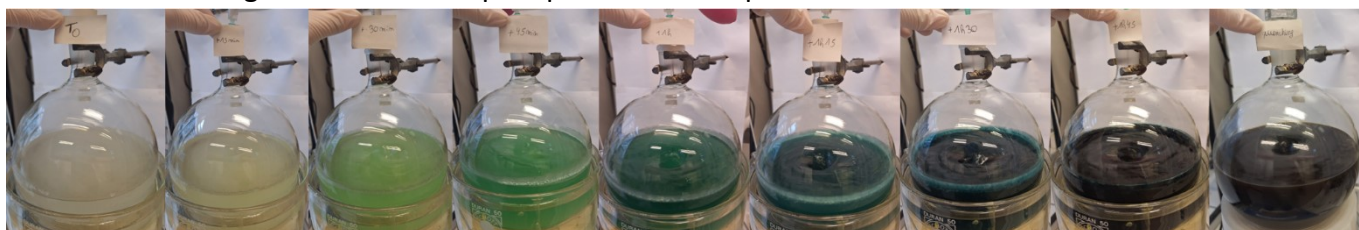
Figure S4. Color evolution of the reaction for the 30 g scale synthesis of P[6]OEt in DCM, 30 °C (0 min., 15 min., 30 min., 45 min., 1h00, 1h15, 1h30, 1h45, quenching with MeOH).
