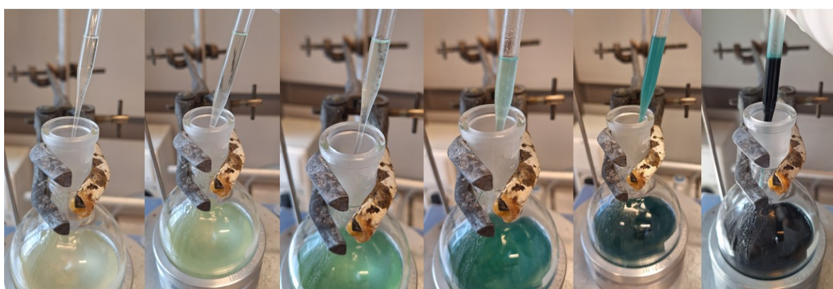
Figure S2. Color evolution of the reaction for the 1 g scale synthesis of P[6]OEt in DCM, 30 °C (from left to right: 15 min., 30 min., 45 min., 1h00, 1h15, 1h30).
