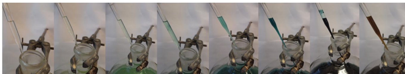
Figure S5. Color evolution of the reaction for the 30 g scale synthesis of P[6]OEt in DCM, 30 °C (15 min., 30 min., 45 min., 1h00, 1h15, 1h30, 1h45, quenching with MeOH).
