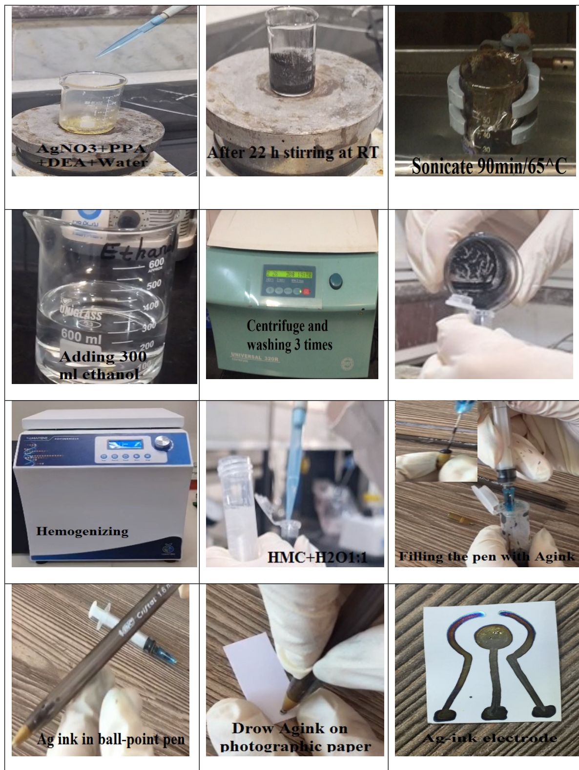
Figure S1. Photographic images of Ag nano-ink preparation procedure.
