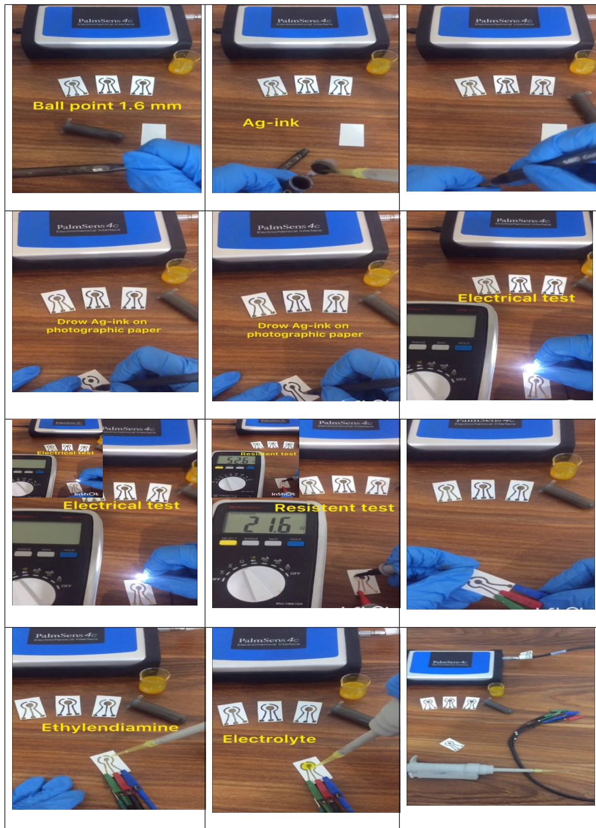
Figure S2. ED A analysis using photographic paper-based sensor.
