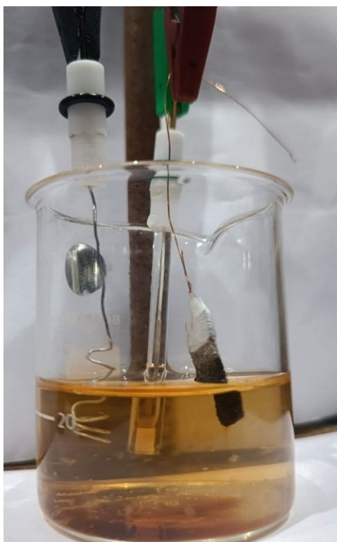
Figure S17: Digital image of performed EC on CQDs and CdSe physical mixture as electrode and a visible leaching of material was observed.
