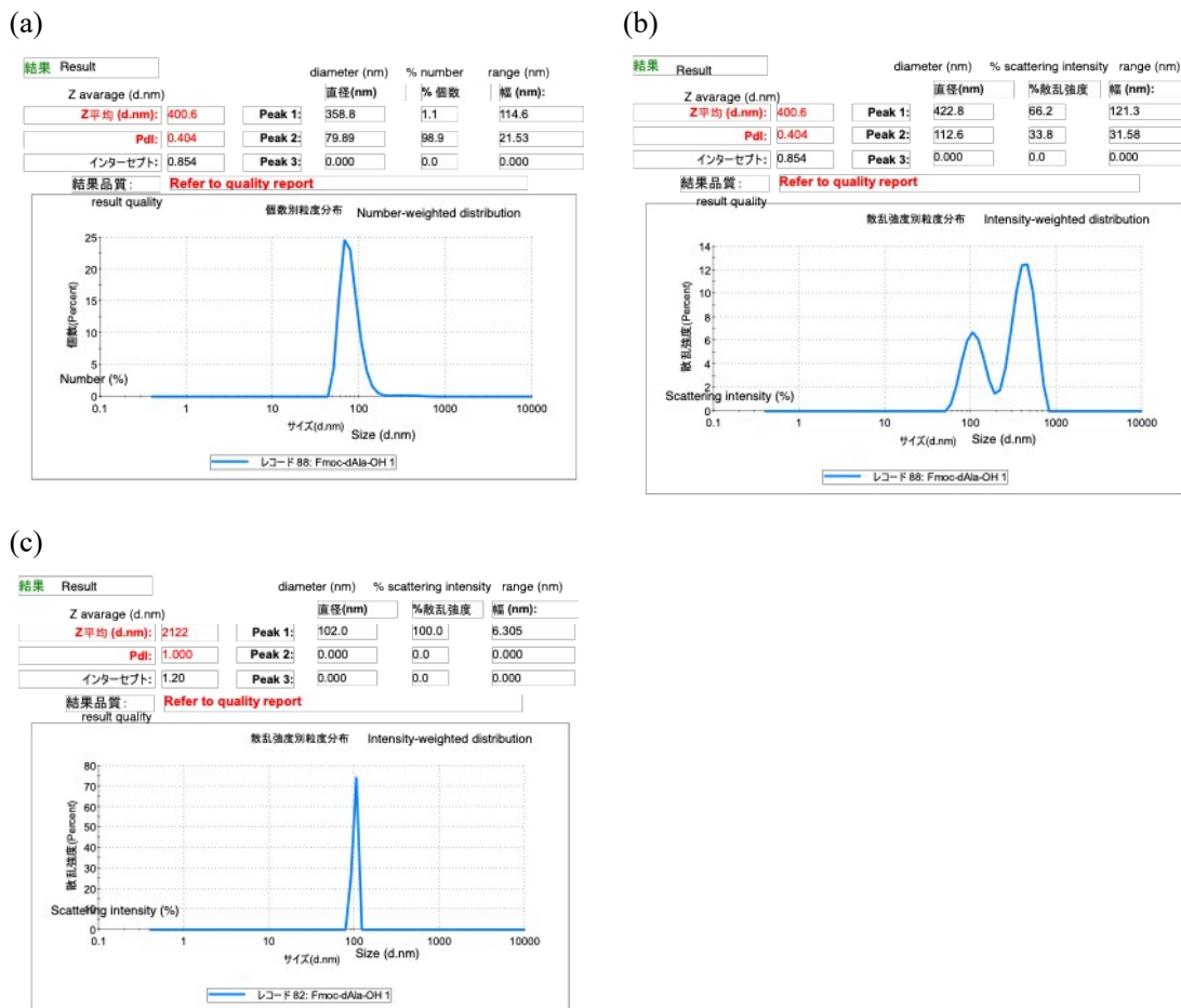
Figure S1. (a) Particle size distribution (number-weighted) for nanoassemblies of Fmoc-DAla-OH with TBTU and DIEA; (b) Particle size distribution (intensity-weighted) before ultrasonication; (c) After 5 min ultrasonication, the intensity-weighted distribution.
