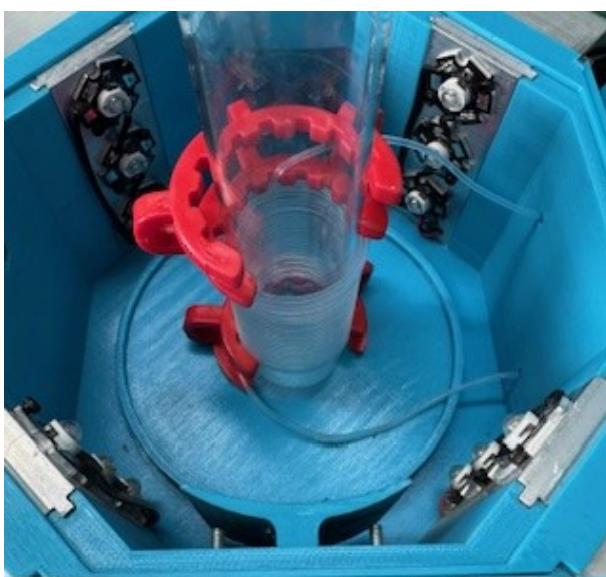
Figure S2. Setup of FEP tube microreactor, during reaction reactor is covered with plastic lid
