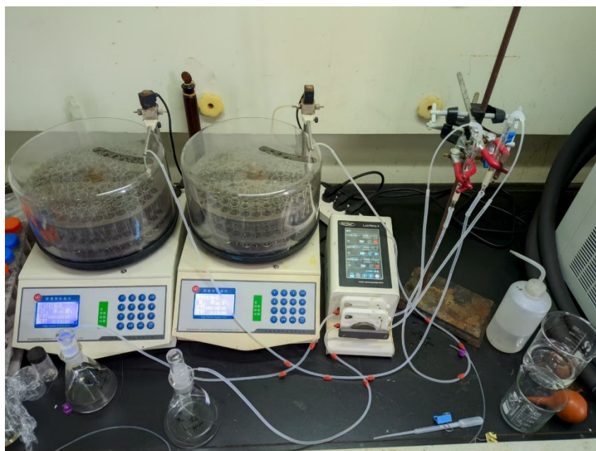
Fig. S6 Column experiment equipment of U(VI) separation by microbial beads
