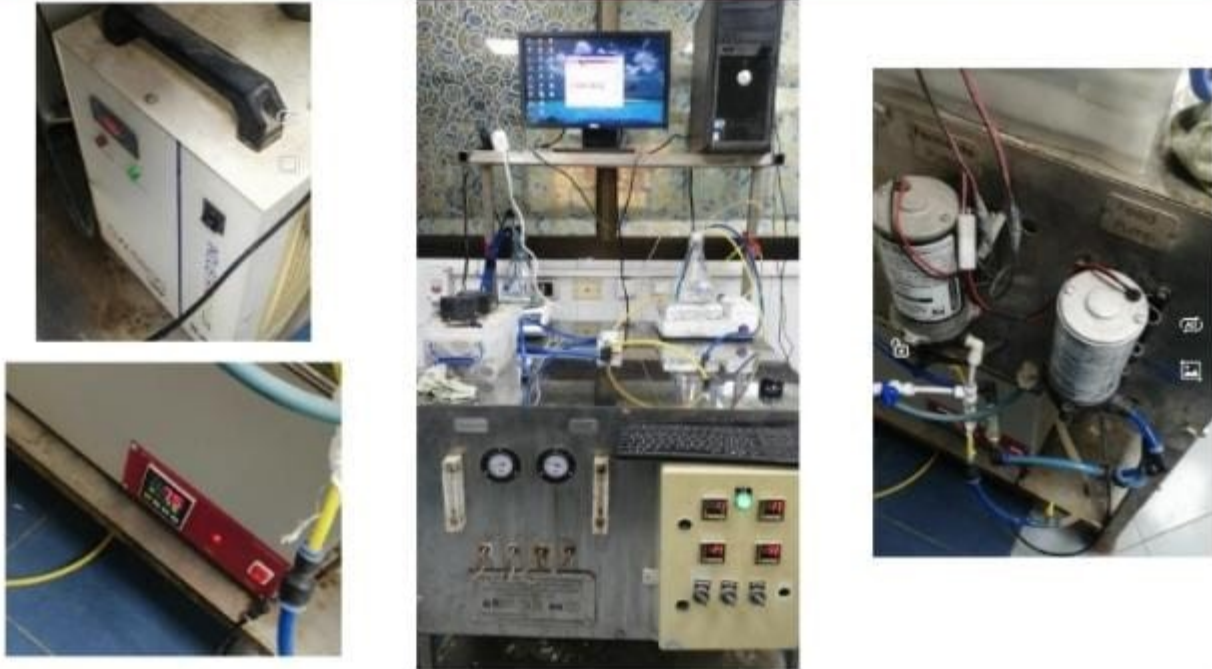
Fig.S2B. Lab Set up of the direct contact membrane distillation (DCMD) apparatus used for photothermal testing under simulated solar illumination.
