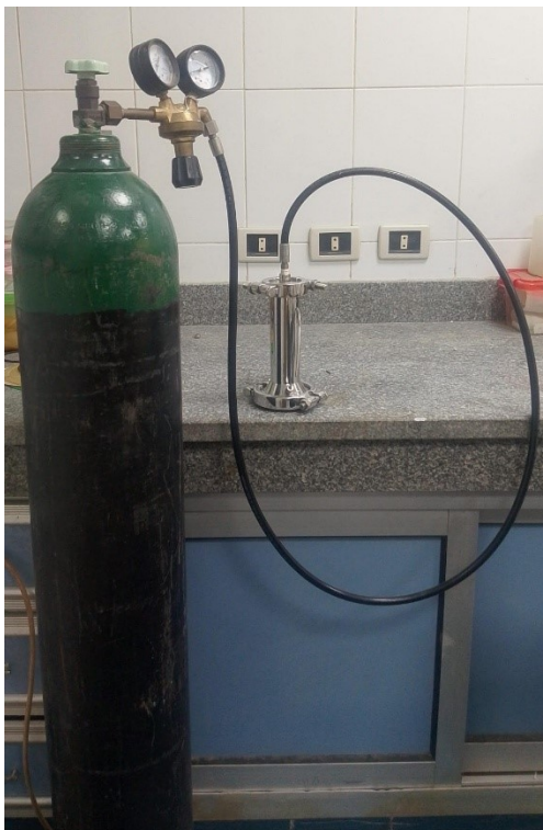
Fig. S1. The Dead-end filtration apparatus for LEP measurement
