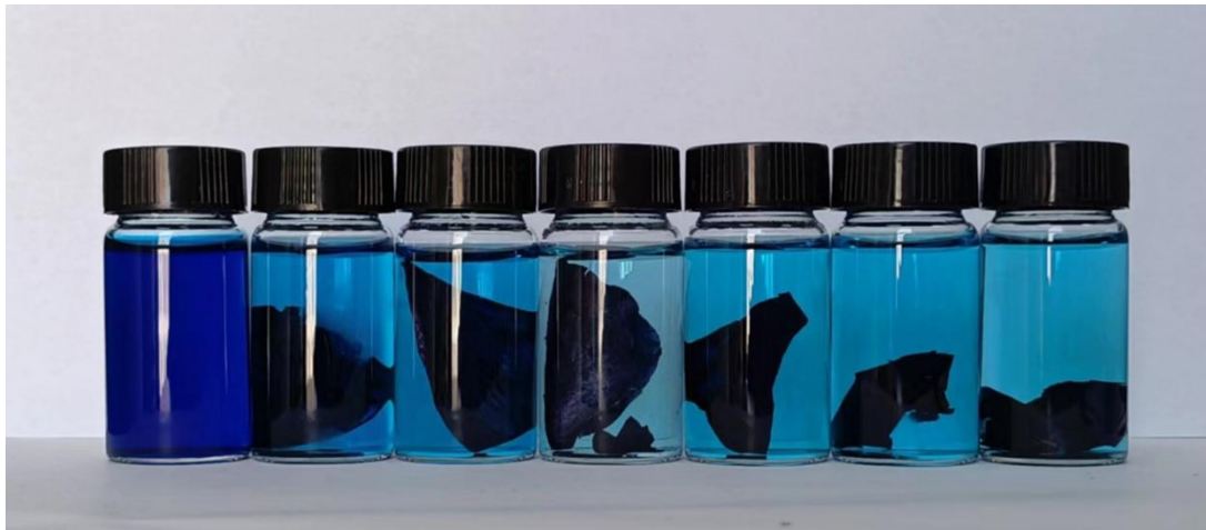
121 122 Fig. S4. Effect of different MXene content in intact membranes on MB adsorption. 123 From left to right: MB without membrane, MB with GO membrane, MB with 124 GO/MXene-10% membrane, MB with GO/MXene-20% membrane, MB with 125 GO/MXene-40% membrane, MB with GO/MXene-60% membrane and MB with 126 GO/MXene-80% membrane.
