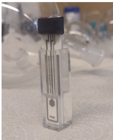
Figure S15. The Pine Research Honeycomb spectroelectrochemistry cell used in this study. The quartz cuvette has a 1.7 mm pathlength. The patterned “honeycomb” electrode is Pt-based, and an external Ag/AgCl reference electrode was also used.
