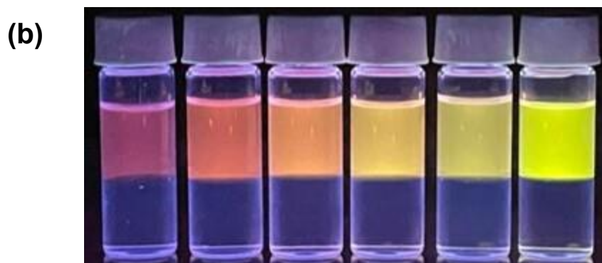
Figure S33 (a) Emission spectra of 2 ( 6.23 \mu\text{M} ) in 70% n -hexane- \text{CHCl}_3 (2 mL) after extraction with different concentrations of PFBA in 4M NaCl (2 mL). The excitation wavelength is 425 nm. (b) A photograph of 2 ( 6.23 \mu\text{M} ) in 70% n -hexane- \text{CHCl}_3 (2 mL) under UV light source ( \lambda_{\text{ex}} = 365 \text{ nm} ) after extraction with PFBA at various concentration in 4M NaCl (2 mL). The concentration of PFBA in the aqueous phase from left to right: 11 mM, 30 mM, 49 mM, 68 mM, 86 mM, 125 mM.
