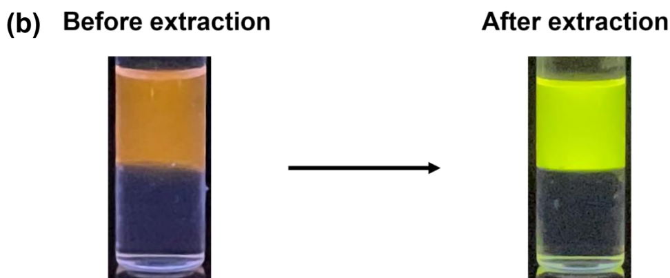
Figure S32 (a) Emission spectra of 2 (6.23 \mu\text{M} ) in 70% n -hexane- \text{CHCl}_3 (2 mL) before and after extraction with PFBA (125 mM) in different aqueous media (2 mL; Red line: D.I. water; Blue line: 2M NaCl; Dark yellow line: 4M KCl; Navy line: 4M \text{Na}_2\text{CO}_3 ). The excitation wavelength is 425 nm. (b) A photograph of 2 (6.23 \mu\text{M} ) in 70% n -hexane- \text{CHCl}_3 (2 mL) under UV-light source ( \lambda_{\text{ex}} = 365 nm) before and after extraction with PFBA in 4M NaCl solution (0.125 M, 2 mL).
