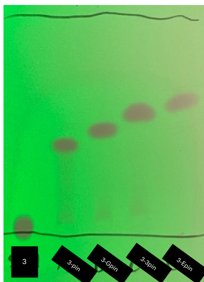
Figure S119. Boronic acid 3 and boronic esters TLC UV analysis using 10% ethyl acetate in hexanes as an eluent.
