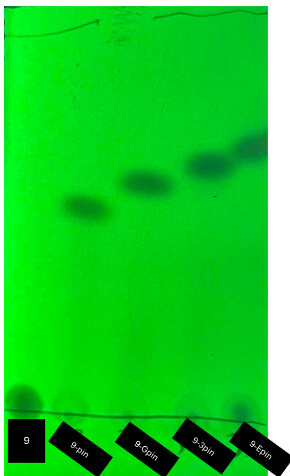
Figure S149. Boronic acid 9 and boronic esters TLC UV analysis using 20% ethyl acetate in hexanes as an eluent
