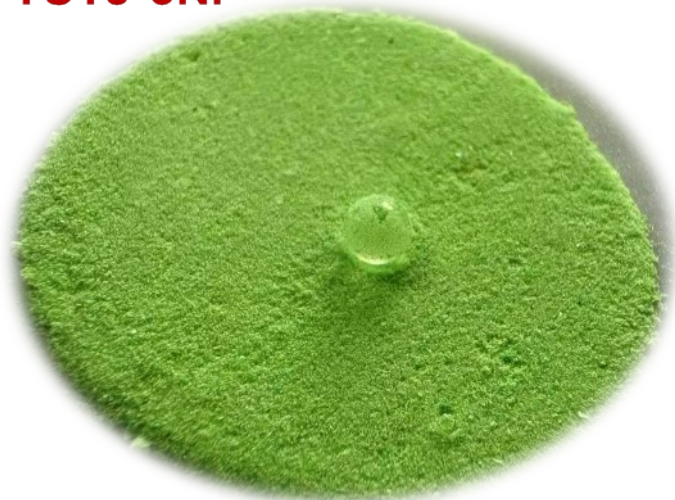
Figure S46. Photograph of a water droplet on a compacted pellet of TUTJ-3Ni.
