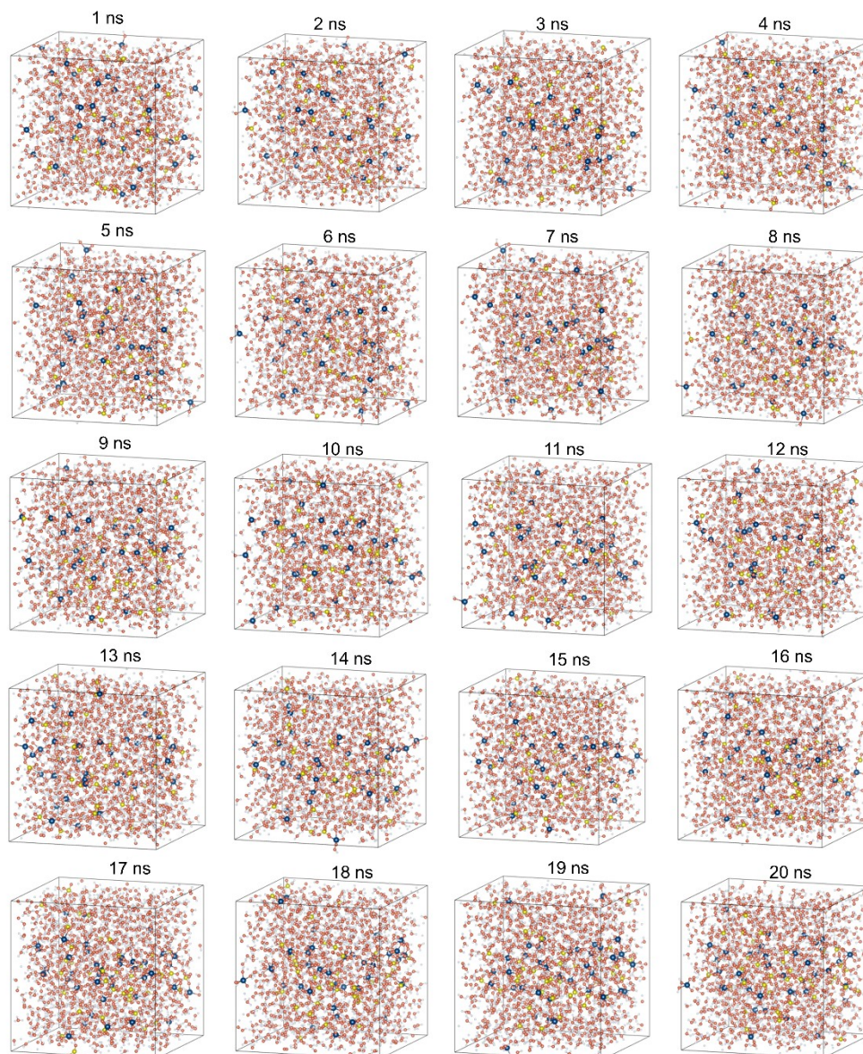
Figure S12. Structural evolution snapshots at 298 K showing configurations at 1 ns interval from 1-20 ns, with vanadium species remaining primarily as small oligomers and large-scale network formation hindered.
