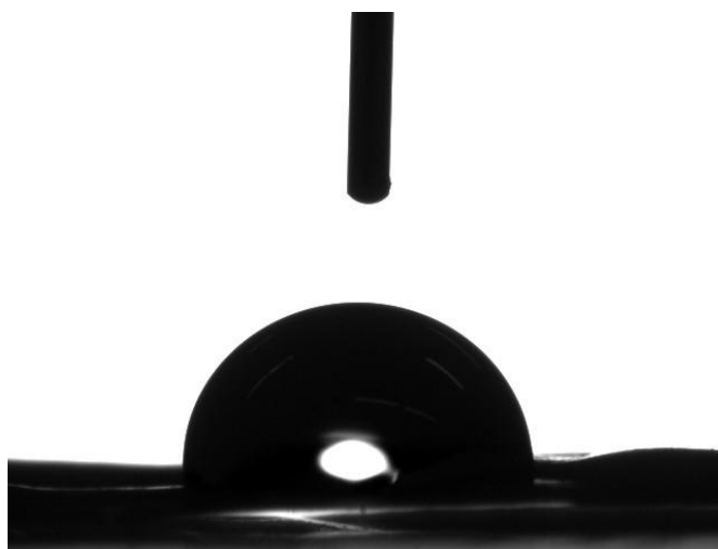
Figure S55. Representative image of a water droplet on nylon-6.6-g-P'BA. The water contact angle was measured at 88 \pm 6^\circ .
