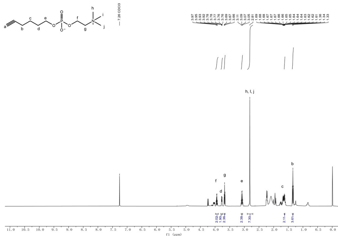
Figure S23. 1 H-NMR spectrum (400 MHz, in CDCl 3 ). 3.92-3.97 (dd, 2H), 3.76-3.78 (t, 2H), 3.66-3.69 (s, 2H), 3.05-3.11 (dd, 2H), 2.81 (s, 9H), 1.61-1.64(m, 2H), δ=1.33-1.36 (t, 2H).
