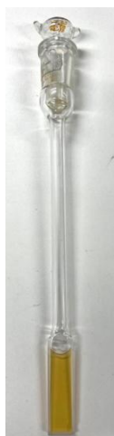
Figure S13. Photograph of the optical cell with a Clear Mating Plug for spectroscopic analysis.
