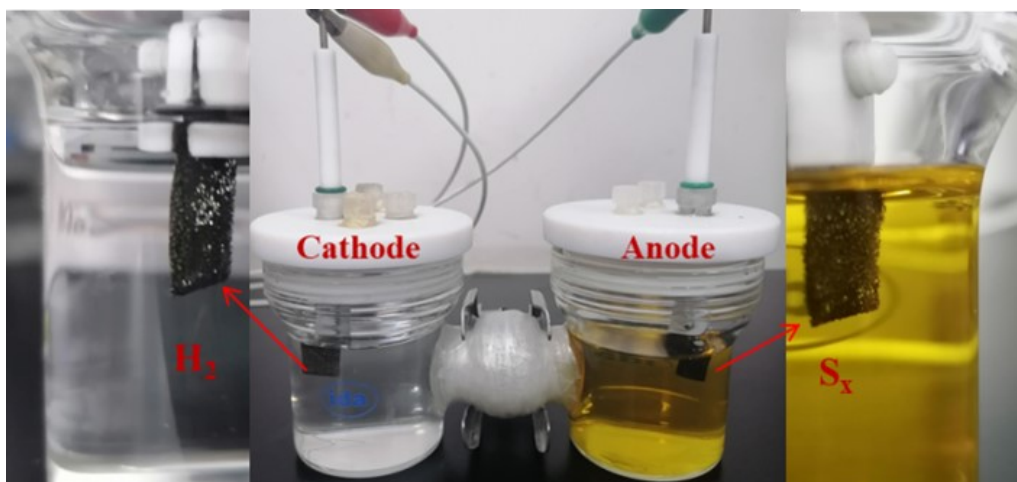
Fig. S38. Digital image of the electrocatalytic coupling system using bifunctional FeCoNiMnMg-S electrodes in 1.0 M NaOH for HER (left) and in 1.0 M NaOH + 3 M Na 2 S for SOR (right).
