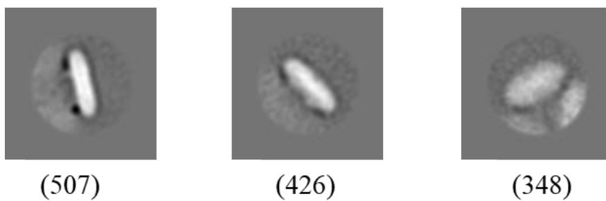
Figure S10. Negative-stain TEM 2D class averages of PSI-PtNP. Numbers in parentheses indicate the number of particles contributing to each class-average image. A total of 1,281 particle images extracted from 65 micrographs were classified into three classes in RELION, followed by 2D class averaging.
