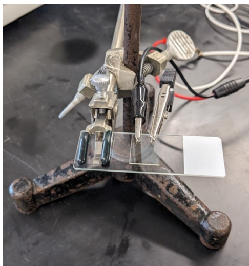
Figure S7. Photograph of an apparatus used to apply electric fields on sample droplets placed on an interdigitated electrode (on the right).
