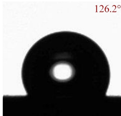
24 25 Fig. S2. Image of the contact angle on a smooth surface after fluorination treatment.
