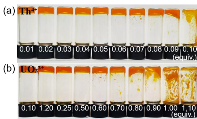
Fig. S29 (a) The effect of adding different equivalents of Th 4+ to a 3 mM ( S )-BINAB solution in i -PrOH/13.5 mM HNO 3 (pH = 1.9) mixture (1:1, v/v) (b) The effect of adding different equivalents UO 2 2+ to 3 mM ( S )-BINAB in i -PrOH/13.5 mM HNO 3 (pH = 1.9) mixture (1:1, v/v) (The numbers at the bottom represent the equivalents of Th 4+ or UO 2 2+ ions).
