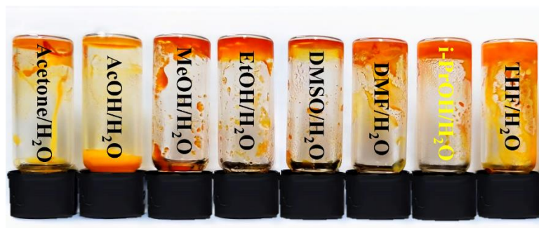
Fig. S16 Gelation properties of ( S )-BINAB in different solvents mixed with water (1:1, v/v) ([( S )-BINAB] = 8 mM)
