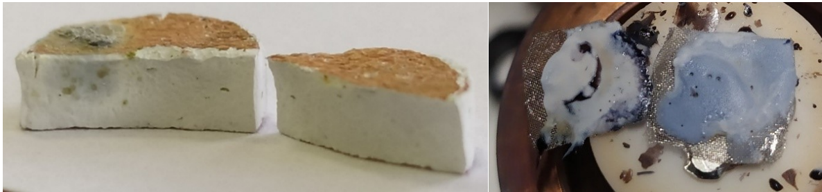
Figure S14. Images of LATP pellets after flash sintering: LATP-4A-100kHz (left, Au electrodes) and LATP-300V-500kHz (right, Pt electrodes).. The observed melting and redistribution of the Au/Pt electrodes, including metallic globules trapped within the ceramic matrix, indicate localized overheating during flash and support the occurrence of temperatures above the melting points of Au (1064 °C) and Pt (1768 °C).
