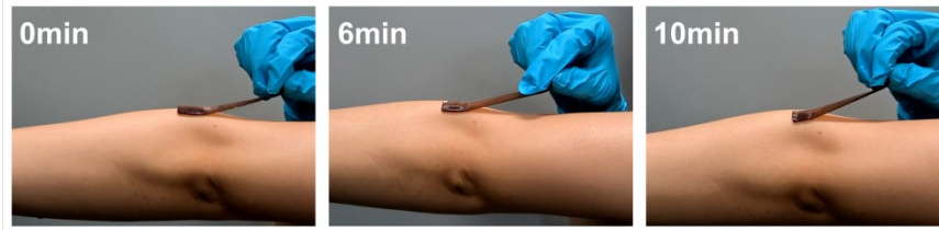
Figure S14. Adhesion photographs of the hydrogel at 0 min, 6 min, and 10 min after the start of "jumping" exercise.
