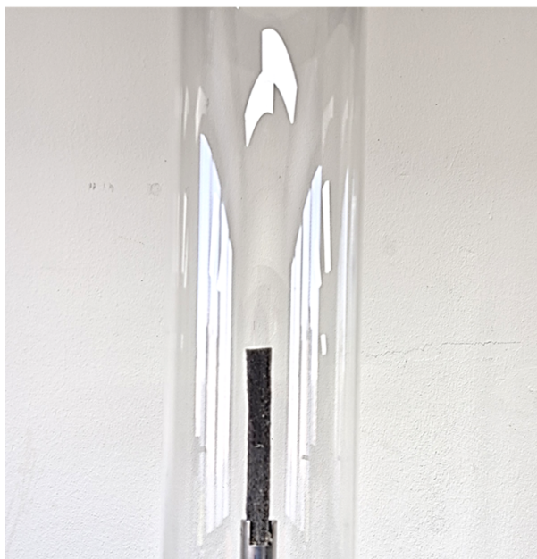
Fig. S10. Photographs of RNA-PUF before and after conduction of LOI test.
