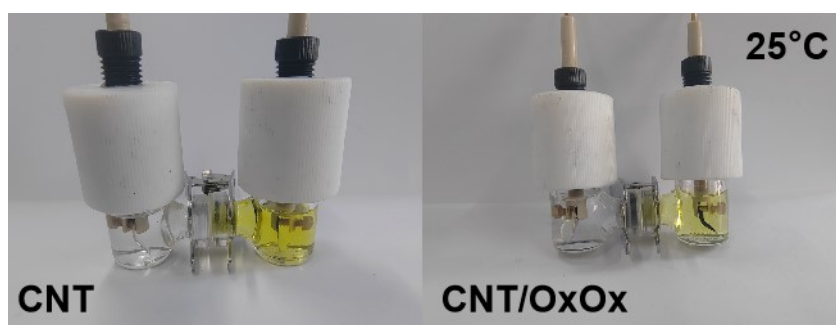
Fig. S18 Digital images of different electrodes after 1 h of discharge in an H-type cell at 25°C.
