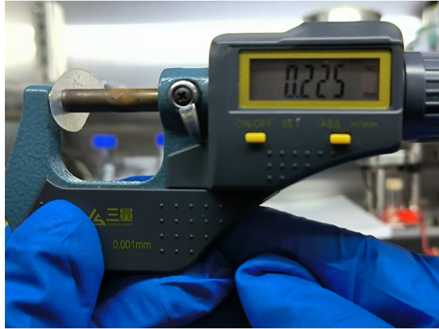
Figure S8. Digital photos of the CPE's thickness measurement by using micrometer. The thickness of the PEO-LiTFSI-Li 3 InCl 6 CPE sample is 225 \mu\text{m} .
