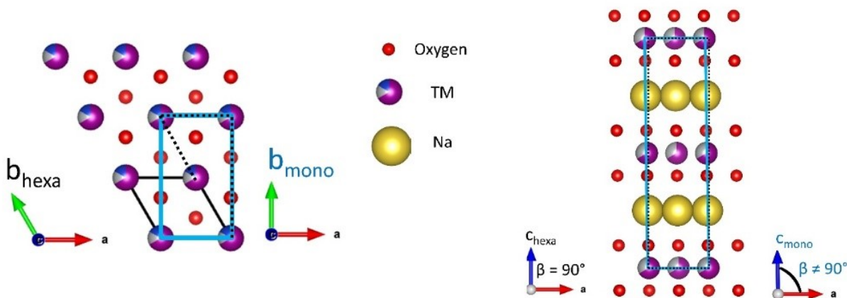
Figure S6. Comparison of hexagonal and monoclinic unit cell representations (left) in the a – b plane and (right) in the a – c plane. Since different space groups have been used, corresponding to different unit cells, the values for the C2/c space group used for P2MnNi and P2MnCu are transformed into the hexagonal unit cell for comparative purposes by applying the following transformation: a_{hexa} = a_{mono} , b_{hexa} = \frac{1}{2}\sqrt{b_{mono}^2 + a_{mono}^2} and c_{hexa} = c_{mono}/\sin(\beta) .
