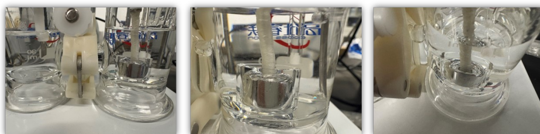
Figure S20. Optical image of the reaction setup with liquid metal as catalyst.
