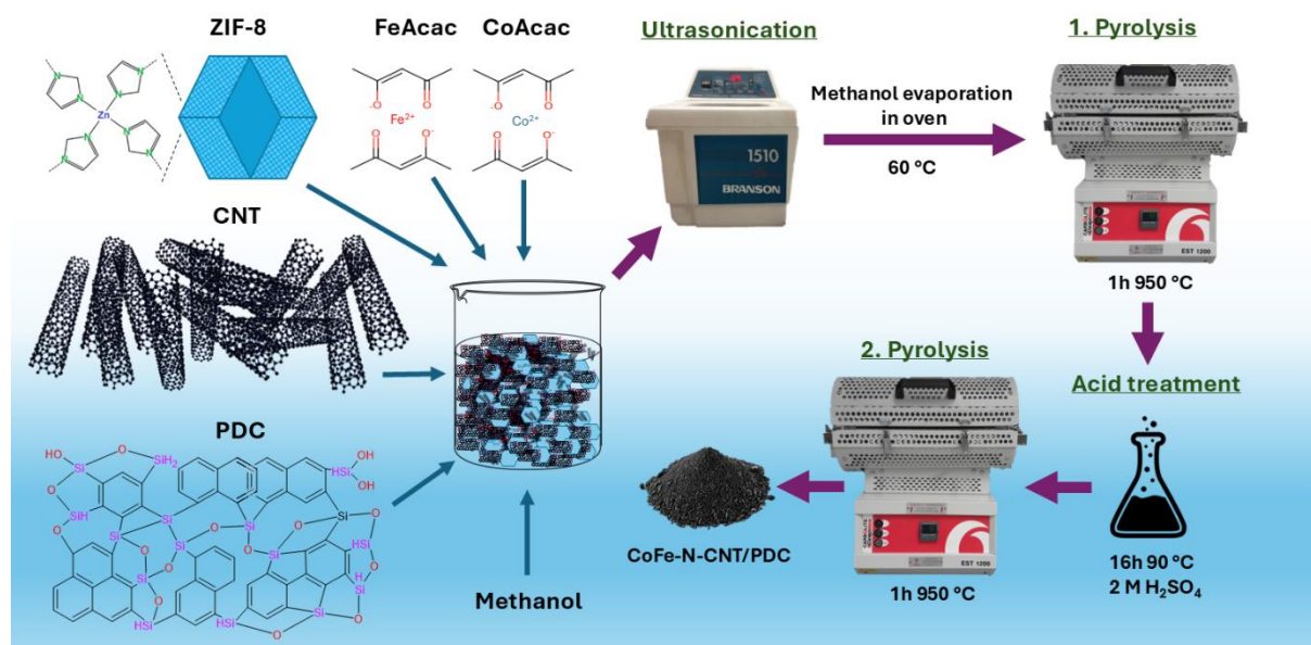
Scheme S1. Pictorial description of the preparation route used for the CoFe-N-CNT/PDC catalyst.
