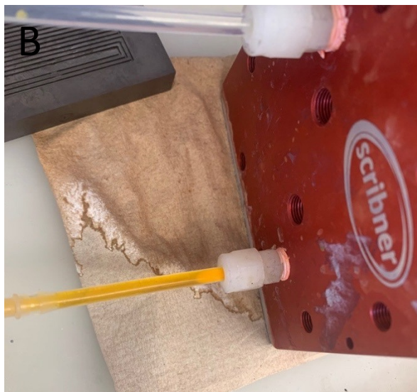
Figure S12. Ce precipitation in flow channel and electrode (A), and clogging of tube (B).
