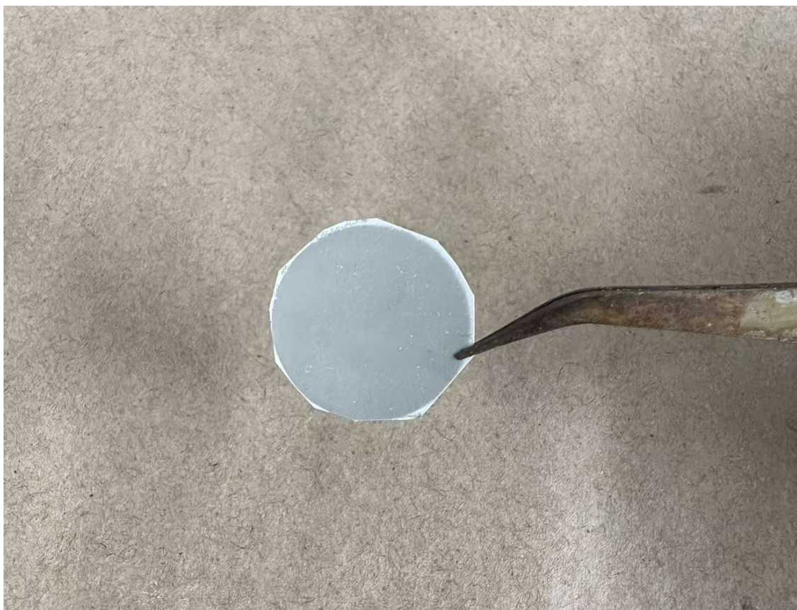
Figure S1. Images of the graphene oxide (GO) membrane (deposition amount: 0.15\text{g}\cdot\text{m}^{-2} )
